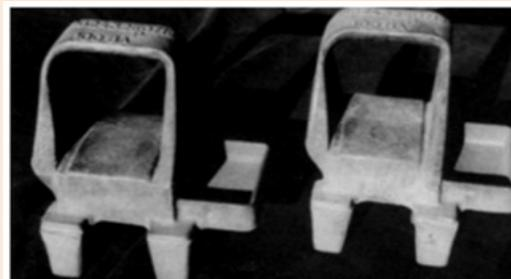
*Cast steel replaced with ADI in truck suspension support*
