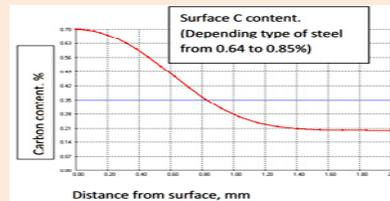
Fig. 1: Example of C profile after case hardening
