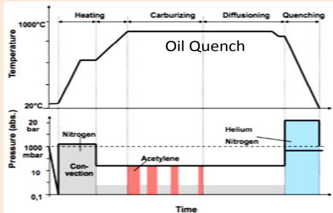
Fig. 3: Low Pressure Carburising Process Cycle
