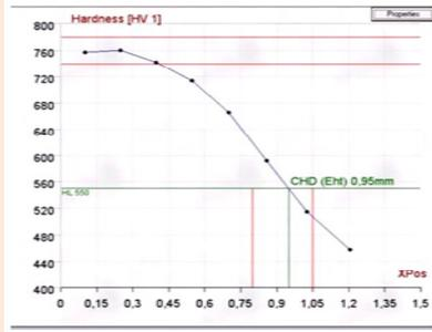
Fig. 2: Hardness profile after case hardening
